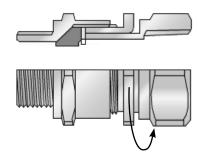
3. Fit the gland into the equipment and fully tighten the Entry Item (1).
