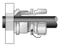
6. Attach the conduit to the Conduit Coupler (5) and fully tighten. Ensure that the Seal Nut (4) does not come loose during this process by holding it with a spanner.
