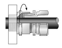
4. Determine the conductor length required to suit the installation and prepare the cable accordingly, removing part of the outer sheath where required to reveal the insulated conductors.
